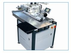
D-PH 510-IX and D-PH 610-IX are an Automatic Pocket Hemming units for jeans and similar sportsware/sportswear. The machine is equipped with a three needle **Kansai** chain stitch sewing head or alternatively a two needle **Brother** lock stitch sewing head. The machine performs the hemming on different fabric types (from heavy to stretch denim) through simple settings witout a change of apparatus or parts. A single adjustable folder allows to single and double hem and change height
